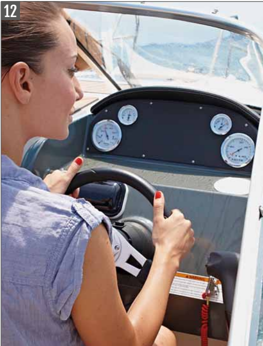
Integrated helm with hydraulic steering, SmartCraft instrumentation, mounting area for 7" GPS/Chart Plotter and 12v outlet
