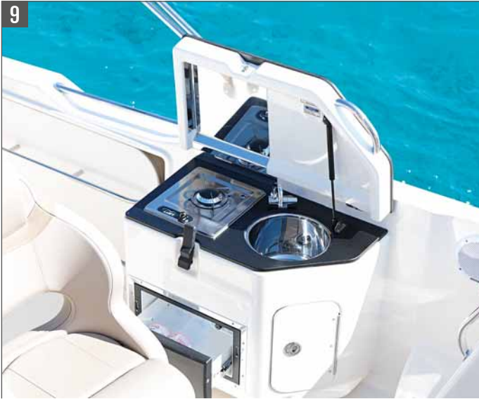
Port galley includes stainless steel sink with cutting board lid, fridge & LPG stove
