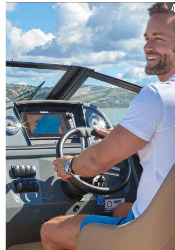
Ergonomic helm with SmartCraft instrumentation with mounting space for 9" GPS/Chart Plotter
