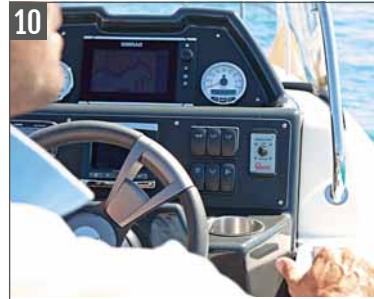
Ergonomic helm with instrumentation and 7" Simrad GPS/Chart Plotter
